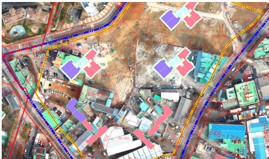
Measurement by Drone – Confirmation of prior interference using overlapped drawings
